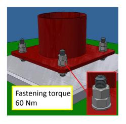
Put one washer and two bolts on each rod and screw them hand-tight.
